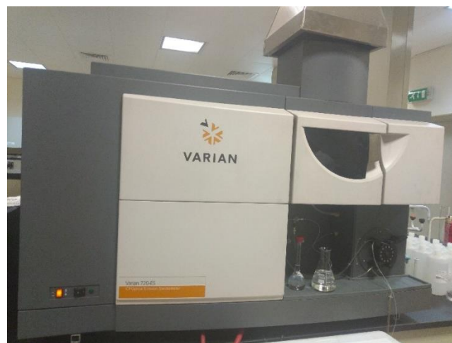
Figure 7: Varian Inductivity Coupled Plasma Optical Emission Spectrometers (ICP- OES) model 720 ES was used for determining the elements through optic waves at different wavelength.
