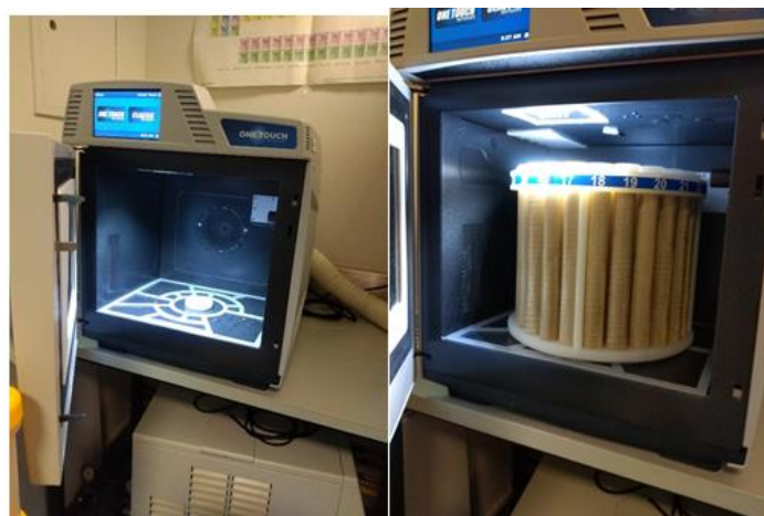
Figure 6: Heating digester One- touch (Mars 6) with the liver samples, was used for breaking down the tissue samples and obtain clear solutions.
