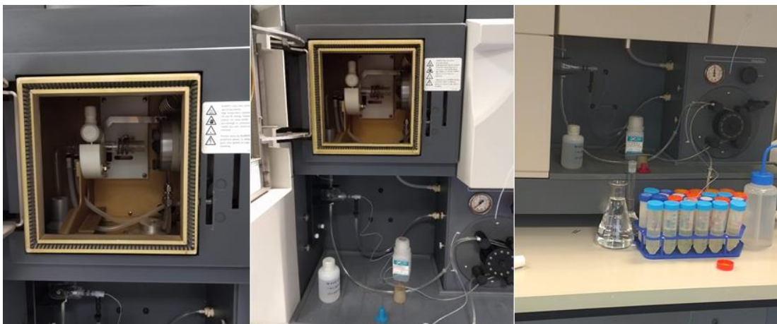
Figure 8: Mechanism of ICP- OES where the samples were allowed to run through the nebulizer for further detection process.
